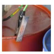
Static grounding clamps must be capable of breaking through coatings, product deposits and rust to ensure a good electrical connection to process equipment.
